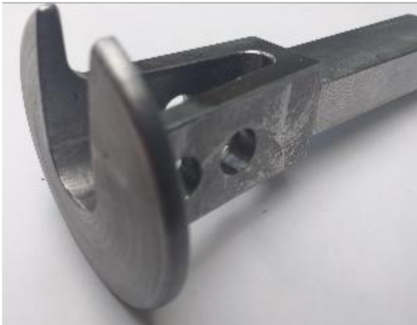
The finished NZR coupling
