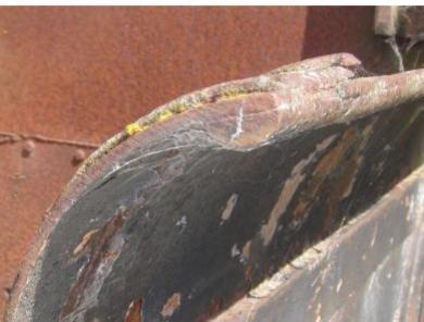
full size beading is 25.4 mm which equates to about 4.5mm on my locomotive and with the limited range of diameters available in these modern times 6.35mm was it but a fraction smaller would have been better.
