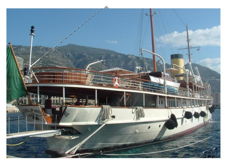
Another point of note is the position of the helmsman. The Captain resides on the bridge (the wooden structure in front of the funnel) but if you look at the stern photograph you can see the tip of the wooden ships wheel controlling the rudder (just in front of the dude wearing the red shirt). The helmsman stands on an open deck at the back of the ship (in all weathers) holding the ships wheel and taking commands from the bridge by telephone.
