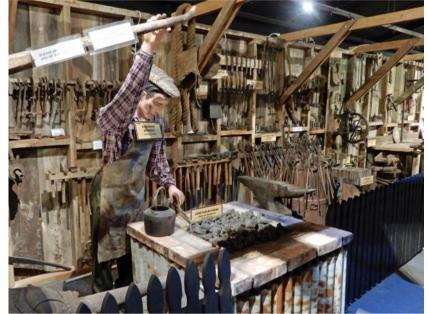
A life size diorama of a blacksmith at his forge swinging on the long wooden lever which operates the bellows supplying oxygen to the burning coals
