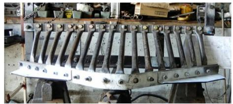
New Cow Catchers are being fabricated for the Wab to the specifications as per the last NZR drawings produced for this item
