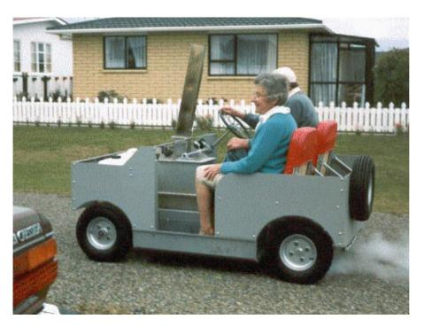
In 1992 I completed a task that had been a dream for many years. This was the building of a steam car. It had a duplex engine with cylinders of 1.625" bore and 2" stroke. The piston valves were actuated by Hackworth/ Marshall valve gear. The mono tube steam generator deliver steam at up to a maximum 600psi.
