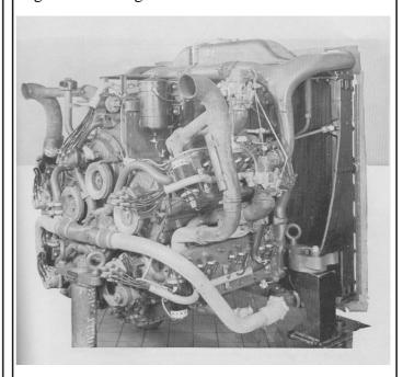
crankcase with each crankshaft driving a common ring gear. One of the immediate advantages was in that tooling for producing the six-cylinder car engine was available for production.
