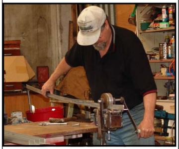
Once each aluminium angle had been rolled it was fitted up onto the steelwork to check the bend radius and to cut to length, deburred and numbered. This process repeated for the smaller section angle, which sat on the larger, spaced apart by the thickness of the Lexan. These were then drilled for the 3/16 pop rivets.
