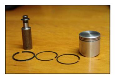
Graeme's piston, rings and the cutter used to cut the slots in the oil ring
