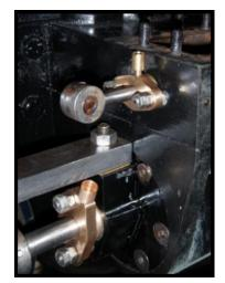
bearing journal but not so the bronze bush in the cross head. Work has also centred on the boiler with new clacks made for the injector and pump feeds to my own design raver than the prototype Kerr Stuart design with flange pipe connections which
