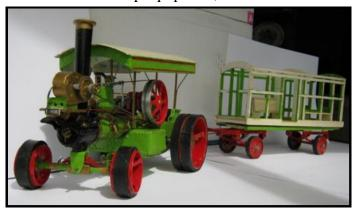
make the model electric powered. The scale chosen was approximately one thirty-second and the model is based loosely on a John Fowler of Leeds 'Showman's engine'. Warick is completing a 'living van' to complement the traction engine. The engine looks very realistic as it trundles along. The owner says that his next project will involve something aligned to live steam.
