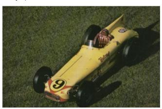
corners on to the long straights, the Ferrari got 'blown away' by the 4 cylinder Offenhauser. The picture is of the Belond Special built by George Salih for the 1957 'Indy 500' which it won. The same car won the 1958 race as well. It was powered by an Offenhauser laid over at an angle of 18 degrees. This was to lower the centre of gravity and give the car a smaller frontal area.
