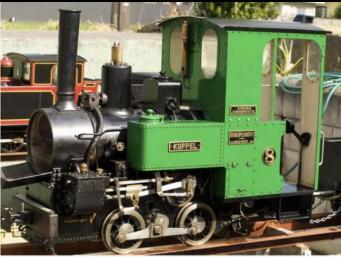
This well-presented Orenstein & Koppel geared locomotive is also fitted with Riggenbach rack gear.
