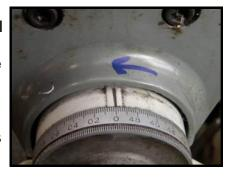
This is so as to be consistent with regard to the backlash in the nut. Not doing so will result in your work inaccurate and possibly having a faster trip to the scrap bin. With the hand wheel dials set on zero at your determined datum edges it is now easy using the graduated dials to accurately position
