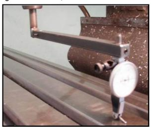
chuck or collet and with a DTI held in the other end (the finger style is best for use with mills). This rotated about the mill table, adjusting the head until the DTI indicates no movement. This can take some time to do so don't move it again. Most of your machining jobs will be done in your
