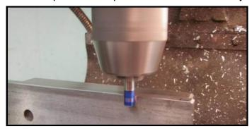
bring the dowel sideways into contact with the jaw so that ink is rubbed off the dowel and left on the jaw. The hand wheel dial is now set to zero and with the quill retracted the table is moved over by half the dowel diameter with the dials reset to zero, this is your datum 0. This process is to be repeated for the other table axis. You could also purchase a wriggler to do
