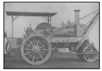
The convertible roller was built by Clayton and Shuttleworth and weighed twelve and a half tons. The engine is a compound with bores of five and a half inches and nine inches and a stroke of twelve inches. There is a boiler feed pump worked by an eccentric on the end of the crankshaft and there is also a steam pump. There are covers over the motion gear, an awning for the driver and a disc flywheel.
