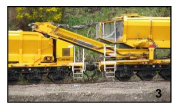
The third picture shows the details of the wagons. Each wagon has a sloped elevator in the floor and material can be moved along onto the next elevator which transfers the material onto the next wagon and so on until all the wagons are filled although the excavator has only been loading the wagon nearest the slip. Each wagon has an operator and a diesel engine powering a hydraulic pump which supplies oil to the oil motors that move the
