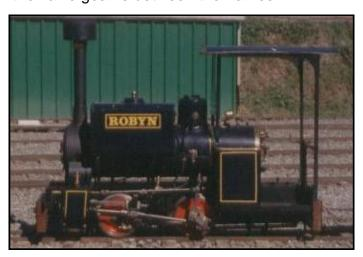
Final Version with inclined cylinders and Hackworth valve gear.
