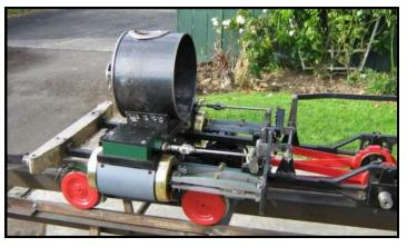
The rear cab supports and cab steps are fitted and the polished brass front and rear cylinder covers are also made and fitted. The smokebox front, door and hinges, and the engine number plate are all completed.
