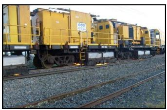
horns and axleboxes wear prematurely. Rail grinding reduces the lifespan of the rail, but the smoother ride greatly reduces the wear and tear on all the rolling stock including locomotives and that more than offsets the cost of early rail replacement.
