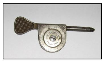
with the counter. Those who work with saws know that the rpm or more importantly the speed of the teeth cutting the wood is absolutely critical. This would be the reason that Disston's made their own rpm counter.
