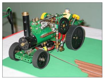
The forward reverse lever operates a switch to control the model.
