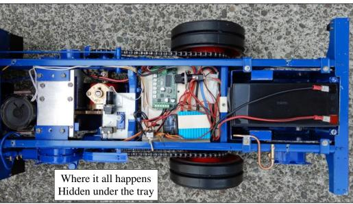
to the body and has chain sprockets fitted to the half shafts. An electric motor bolts between the frames with another gear wheel to drive the differential. 7mm chain provides the drive to the rear wheels. A replica steam engine and gearbox casing covers these components.
