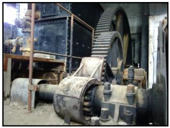
The No 8 on the gold dredge is a statement of its size – 8 cubic feet of gravel per bucket load. This is photo of the gear train driving the bucket elevator of the dredge.
