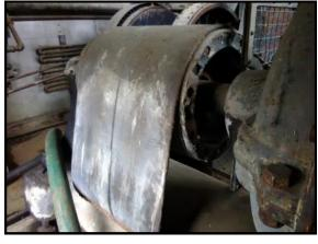
side plates. The whole assembly is turned round before use and provides a compact pulley that can transmit more power than a traditional metal pulley of similar proportions.
