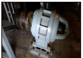
This photo is of a raw hide pulley installed on one of the electric motors. This pulley is fabricated from layers of leather sheets riveted between two iron
