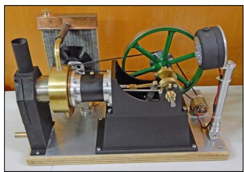
connection to a gas container for heating and a burner canopy to concentrate the heat to the end of the displacer.
