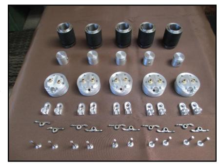
Rocker pivot brackets, pins and valve spring retainers made.
